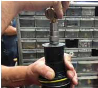
Sprinklers are Rebuilt
